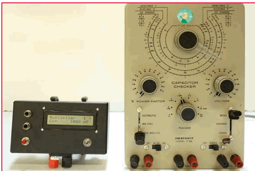
Figure 1. The IT-28 weighs a hefty 5 lbs (2.2 kg) and needs to be plugged in, while the battery powered Pico C-Super is a relative lightweight physically but not in measurement capabilities. The open magic eye shown here occurs when the bridge is balanced.
